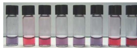
Fig. 4. Color changes of an aqueous solution of 2 (400 \mu L) upon addition of a larger amount of analyte (as sodium salt, 70 \mu L, 0.1 M). From the left: fumarate, maleate, oxalate, malonate, succinate, glutarate, propionate, and 4-pentenoic acid.
